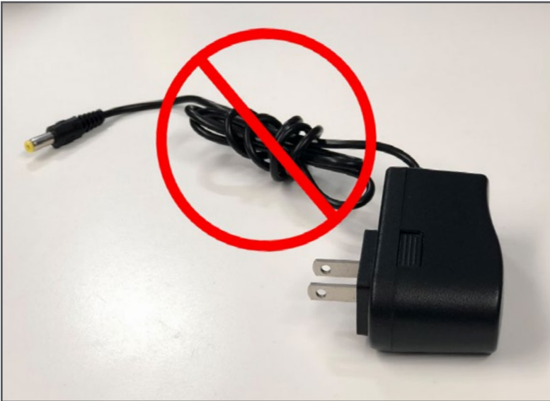
Figure 1: To reduce fire risk, never wrap or bundle wires.
